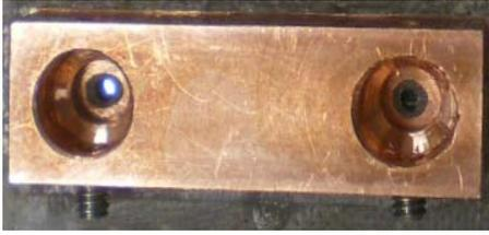
Figure 4: The drilled copper piece for laser diode integration
