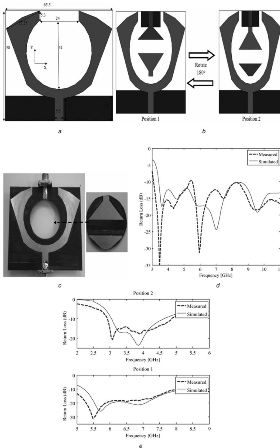
**Fig. 5** The complete rotatable reconfigurable cognitive radio antenna system
