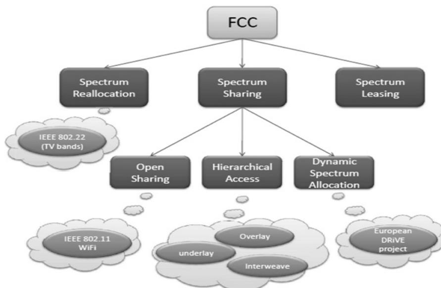
**Fig. 1** Proposed FCC solutions to the spectrum underutilisation
