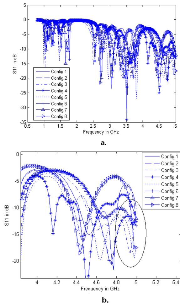
Fig. 3. S11 plot for the antenna in [16] for the configurations presented in Table 1. A) zoomed out, B) zoomed in at 5 GHz
