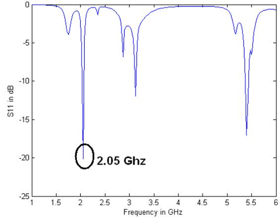
Fig. 11 The antenna's reflection coefficient with backup switch S2 and S3 activated showing clear operation at 2.05 GHz
