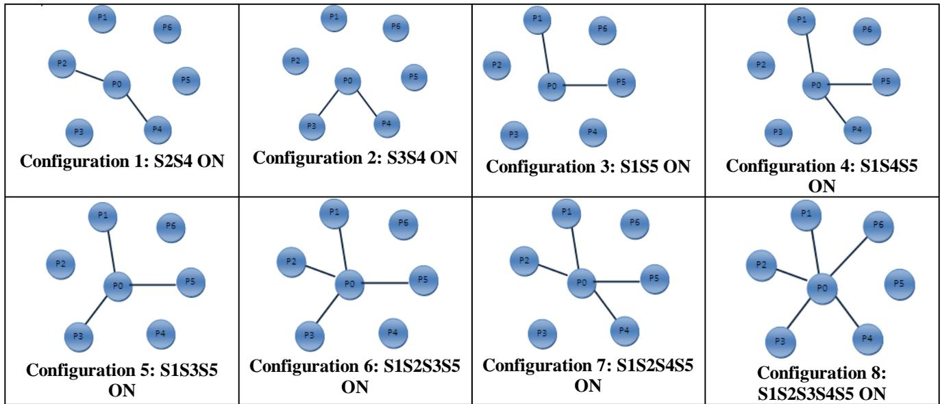
Table 1. The different configurations of the antenna in [15] that lead to operation at 5 GHz
