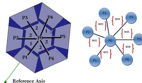
Fig. 2. The antenna in [16] with its graph model
