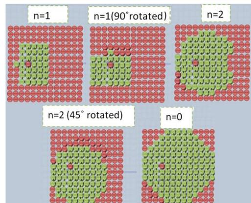
Fig. 7 Graph models for the required antenna configurations ( 5 different modes) – parts in green indicate parts where switches are ON, parts in red indicate switches are OFF
