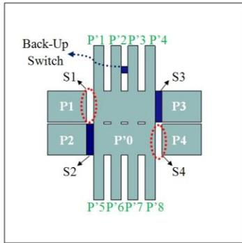
Fig. 9 Antenna using backup switch for 2.05 GHz equivalent configurations
