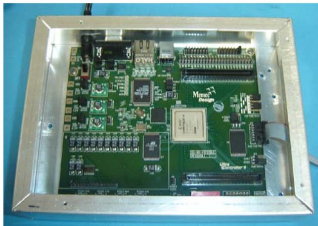
Fig. 1: Xilinx's Virtex-4 FX XC4VFX12-FF668LC Development kit. For testing, the LCD panel was removed and the board was placed in a box, with lead protecting all the components but the FPGA.
