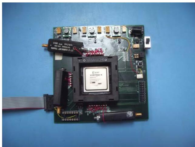
Fig. 2. Custom board design for monitoring photocurrents for the three XC4VFX12 power supplies –  $V_{\text{core}}$ ,  $V_{\text{aux}}$ ,  $V_{\text{I/O}}$ .
