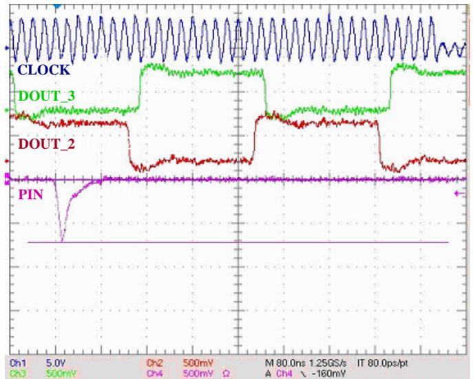
Figure 3. Dose rate response of a commercial XC5VLX50T showing clock drop-out
