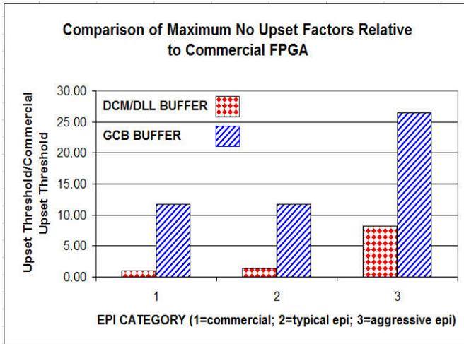
Figure 10. Comparison of maximum no-upset threshold for a commercial bulk silicon substrate and two experimental epi thicknesses
