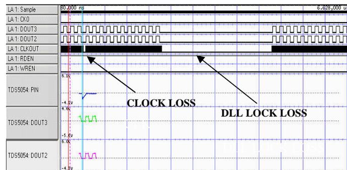
Figure 9. BRAM/FIFO lowest upset threshold showing latent upset characteristic of DCM/DLL.
