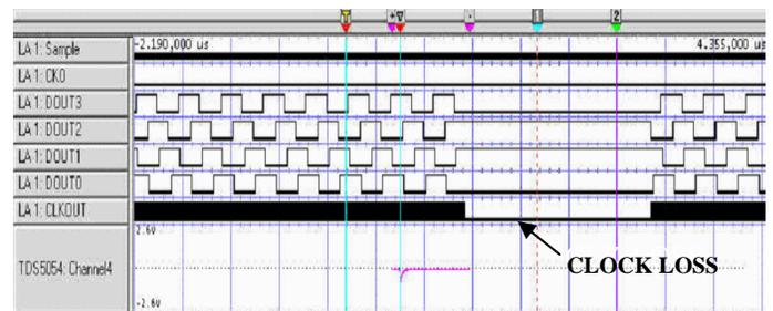
Figure 4. Logic analyzer record of upset shown in Figure 3.
