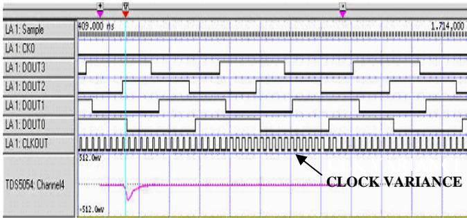
Figure 5. Dose rate response of commercial XC5VLX50T showing a variance in the clock cycle
