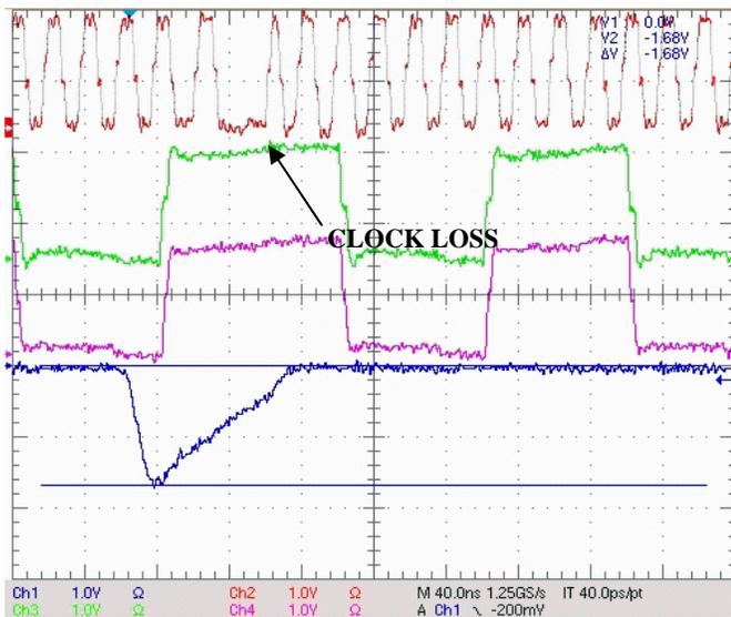
Figure 6. Minimum upset characteristic for BRAM/FIFO using the GCB for clock buffering.
