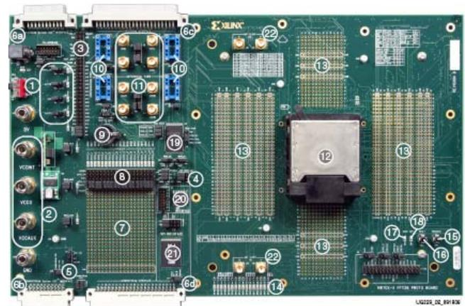
Figure 1. UG229 Virtex-5 LXT Prototype Platform [2]
