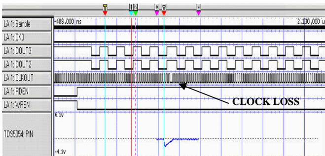
Figure 7. Logic analyzer record for BRAM/FIFO minimum upset characteristic for the BRAM/FIFO.
