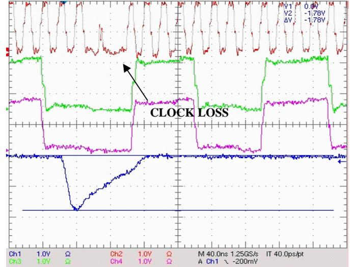
Figure 8. BRAM/FIFO lowest upset threshold showing characteristic GCB upset
