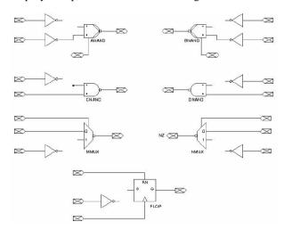
Figure 2. Structured ASIC Primitive Cell
