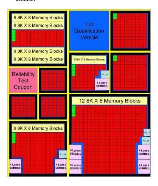
Figure 4. Reticle Floor plan for S-ASIC
