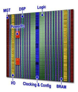
Figure 1: Physical layout of the SIRF chip
