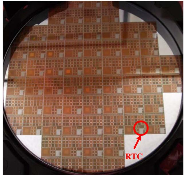
Figure 2. RTC incorporated on an MPW wafer
