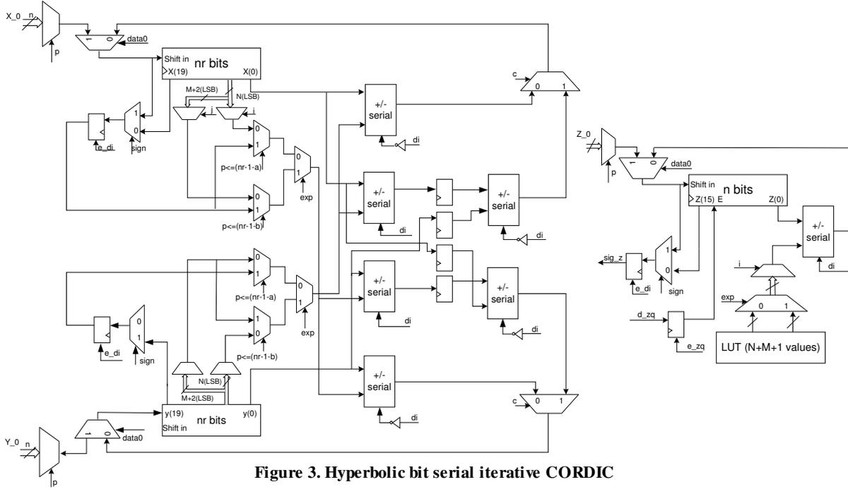
**Figure 3. Hyperbolic bit serial iterative CORDIC**
