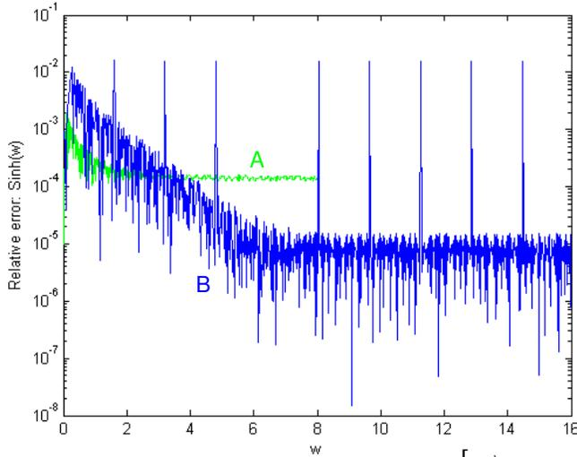
**Figure 10.** In Curve A, 24 bits were used ( $w \in [0,8)$ ). In Curve B, 32 bits were used ( $w \in [0,16)$ ).
