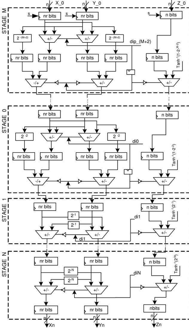
Figure 2. Pipelined-CORDIC
