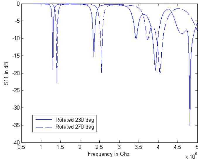
Fig.4. Antenna tuning by rotating the Chebychev slots
