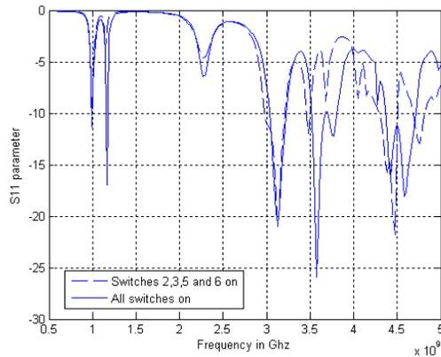
Fig. 4.  $S_{11}$  results when switches 2, 3, 5 and 6 are activated and when all the switches are activated.
