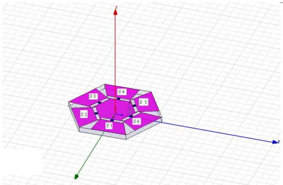
Fig. 1. Geometry of the star antenna showing the different slots and the switches.
