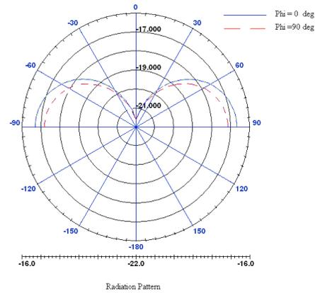
Fig. 6. Radiation Patterns for  $\Phi=0^\circ$  and for  $\Phi=90^\circ$  with all switches activated.
