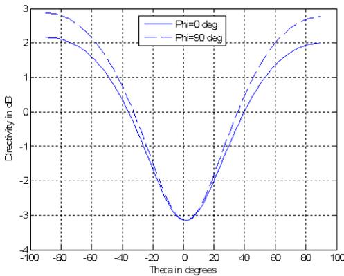
Fig. 5. Total directivity of the antenna as a function of the angle theta.
