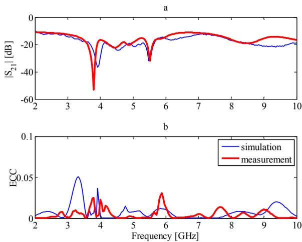
Fig. 5(a) The coupling (b) the envelope correlation coefficient of the antenna
