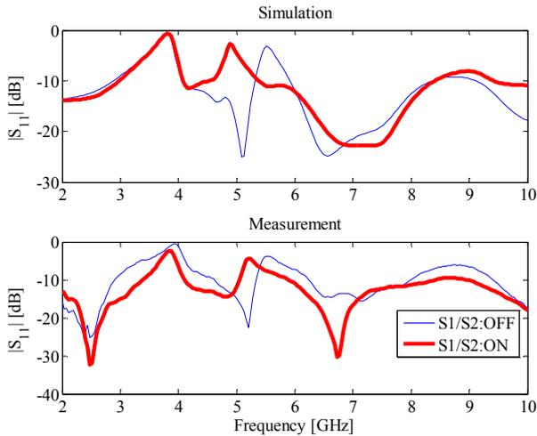
Fig. 4 The simulated/measured reflection coefficient for the MIMO antenna
