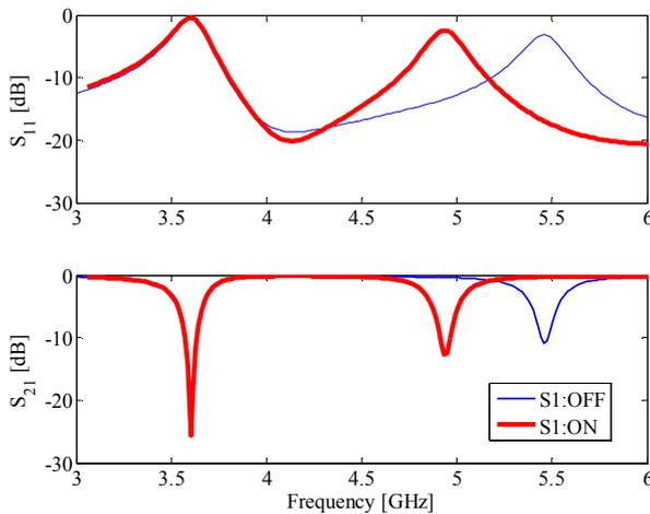
Fig. 2 The filter S-parameter for the two mode of operation of the switch  $S_1$
