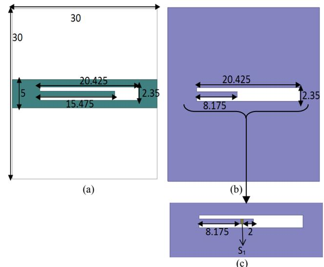
Fig. 1 (a) U-slot in the feeding line (b) U-slot in the ground plane (c) the incorporation of a pin-diode in the U-slot of the ground plane
