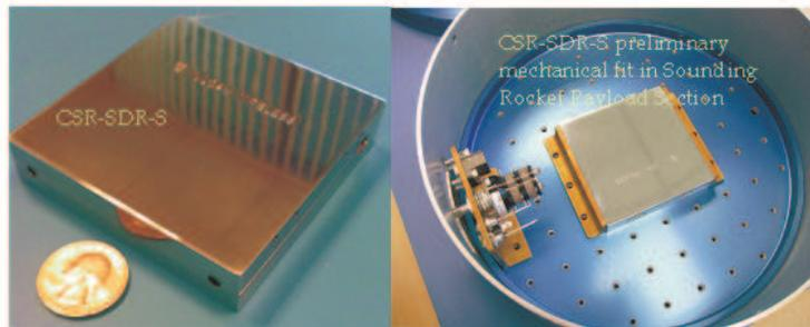
**Figure 2. CSR-SDR-S TDRSS-MA Software Defined Radio and PTS-4 Payload Configuration.** *The view on the left shows the CSR-SDR-S CubeSat radio and the view on the right shows the CSR-SDR-S mounted into the PTS-4 payload housing. Picture by Vulcan Wireless Inc.*
