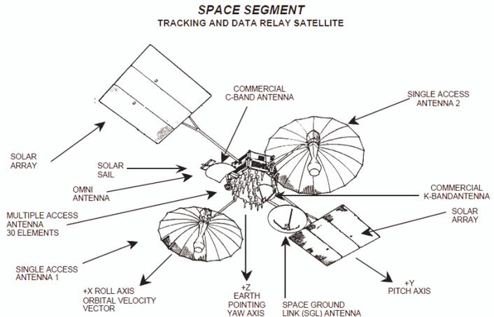
**Figure 1. Tracking and Data Relay Satellite Configuration (F1-F7 Shown).** The multiple access antennas, which are comprised of a 30 element phased array, are shown mounted to the nadir deck of the space craft. [1]
