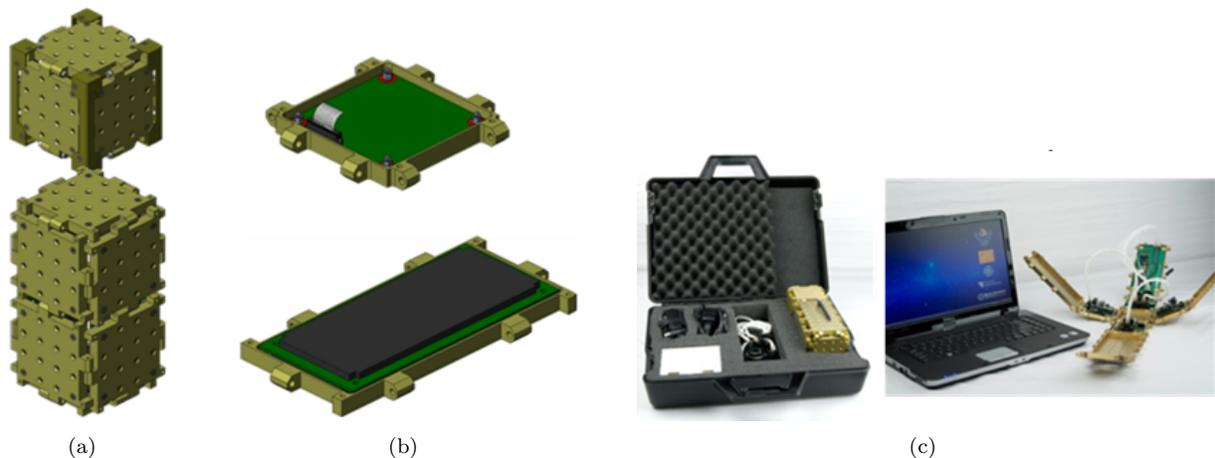
**Figure 2. CubeFlow modular architecture for CubeSats. (a) 1U and 2U CubeFlow examples, depicting peg-board style modular structure concepts. (b) Examples of interchangeable components, employing plug-and-play interfaces and the CubeFlow structural format. (c) Cubeflow development kit, featuring CubeFlow structures, integrated spacecraft computer, interface modules, and development tools.**
