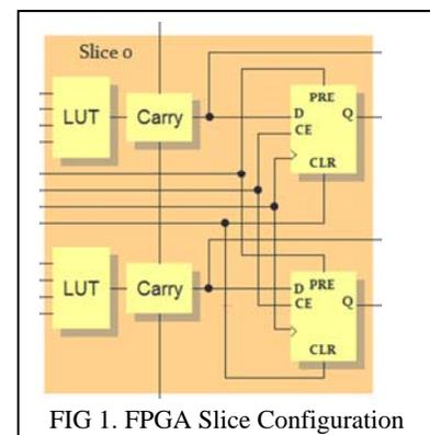
FIG 1. FPGA Slice Configuration
