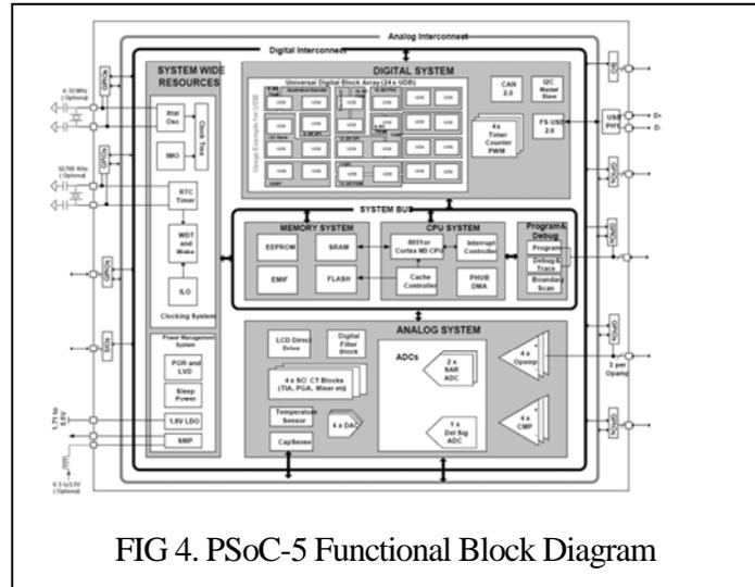
FIG 4. PSOC-5 Functional Block Diagram
