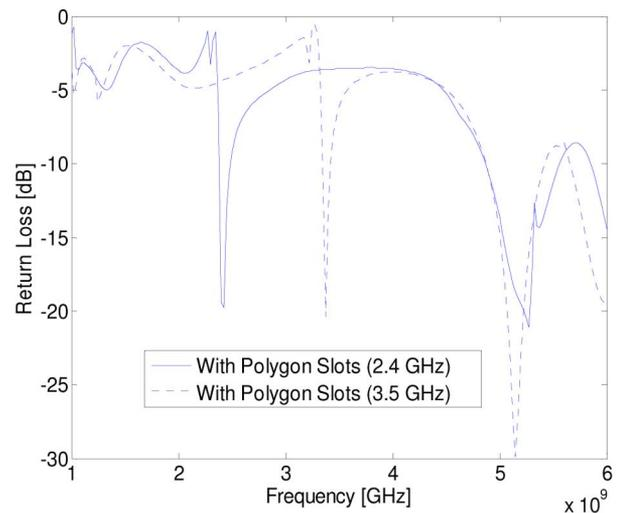
Fig. 6. S11 plot for the case of the slots in the form of a polygon.
