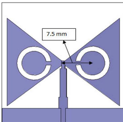
Fig. 3. Antenna structure for the case of circular slots.
