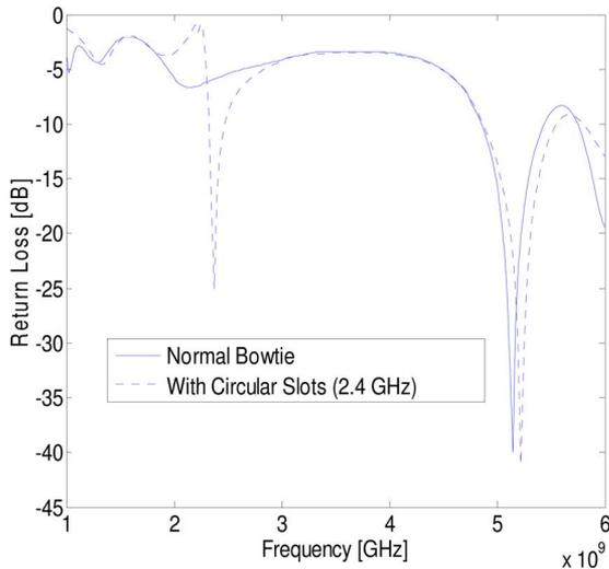
Fig. 2. Return loss for different antenna designs.
