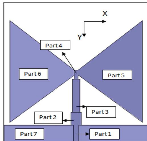
Fig. 1. First antenna design.
