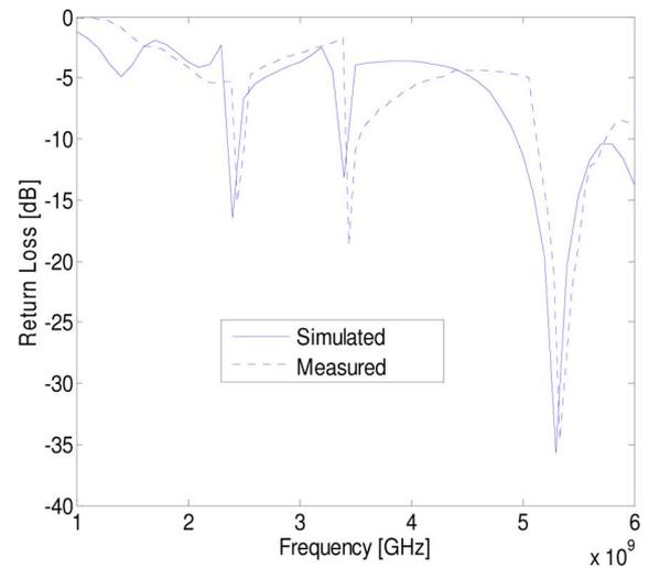
Fig. 8. Simulated and measured S11 plot.
