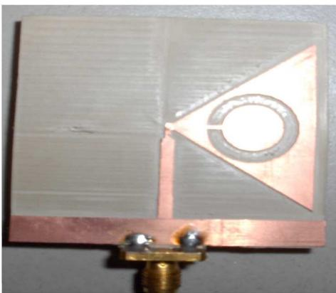
Fig. 7. (a) Final bowtie design. (b) Fabricated top side. (c) Fabricated bottom side.
