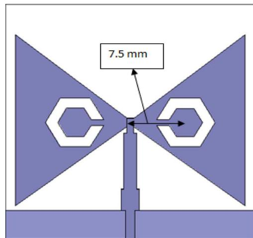
Fig. 5. Antenna structure with slots in the form of a polygon.
