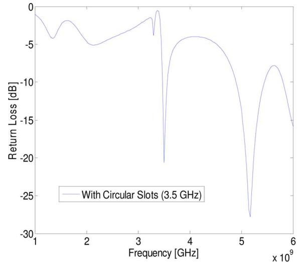
Fig. 4. Return loss for the case of circular slots.
