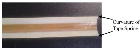
Fig. 3. Dipole with the actual composite tape-spring.
