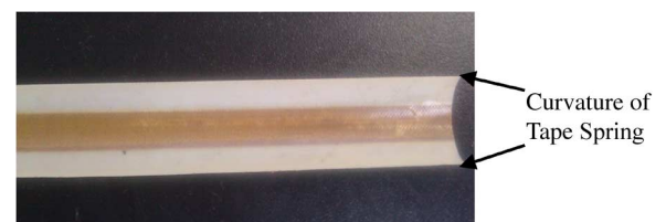
Fig. 3. Dipole with the actual composite tape-spring.
