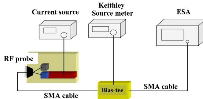
Fig. 6. Apparatus of the RF signal measurement.
