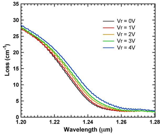
Fig. 3. Room-temperature total loss spectra of the QDMLL device as measured by the multisection technique.
