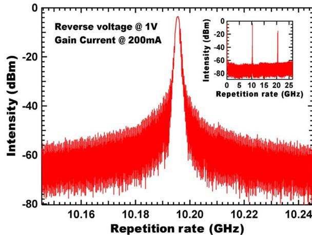
Fig. 8. RF power spectrum of the electric pulse signal directly extracted from the saturable absorber. The resolution bandwidth: 1 MHz.
