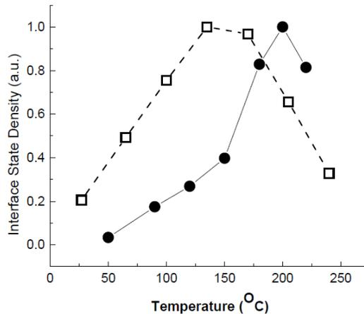
**Figure 3** Temperature dependence of the interface trap density for NBTI (solid circles) and radiation effects (open squares).
