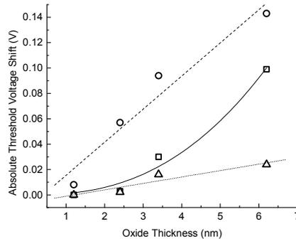
**Figure 2 Thickness dependence of threshold voltage shifts.**
