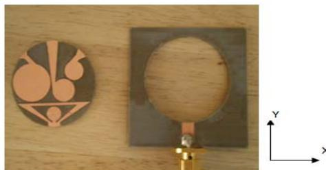
Fig. 2. (a) The different shapes for the same antenna structure (b) The fabricated prototype
