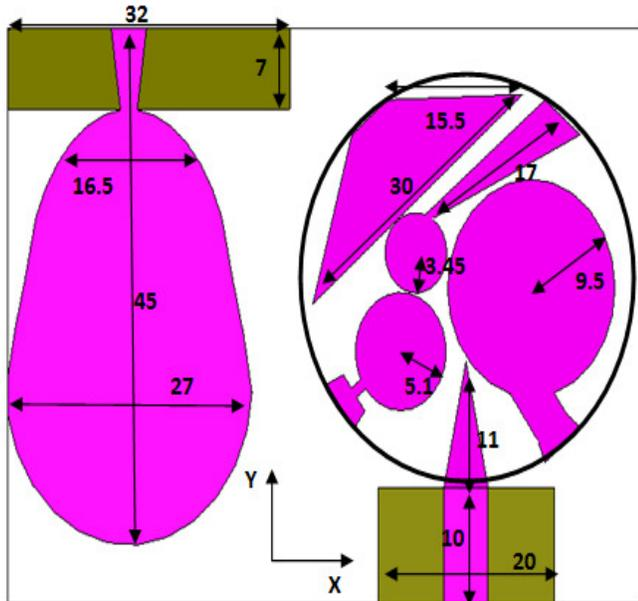
Fig. 1. The antenna structure (dimensions in mm)
