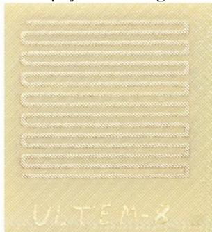
**Figure 7. Passive Test Circuit after outgas testing**
