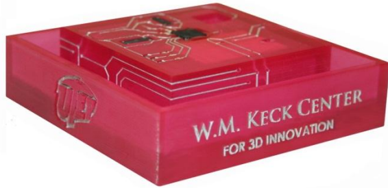
Figure 4. CubeSat Control & Data Handling Module Proof of Concept.
