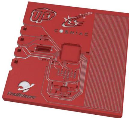
**Figure 5. CubeSat Facet AT90USBKEY Proof of Concept.**
