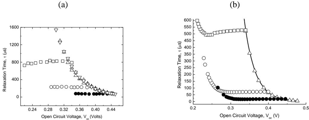
Figure 1: The experimental (a) and simulated (b) relaxation times as a function of the open circuit voltage. Triangles ( $\Delta$ ,  $\nabla$ ) are the results where  $V_{oc}$  is varied by changing the light level/generation rate. Squares, open circles, and solid circles are the results when  $V_{oc}$  is changed by irradiation(a)/adding trapped hole charge(b).
