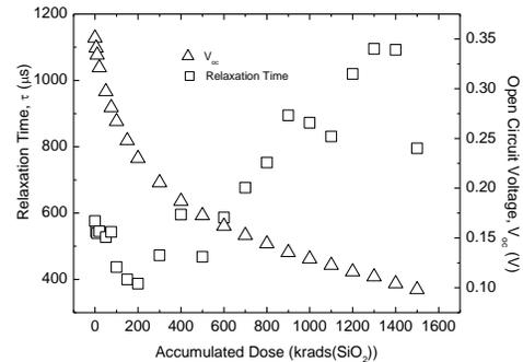
Figure 3: The relaxation time and a open circuit voltage as a function of the accumulated dose when the light level produces a  $V_{oc}=0.35$  V background before irradiation.
