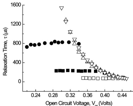
Fig. 1. The experimental relaxation times as a function of the open-circuit voltage. ( $\Delta$ ,  $\nabla$ )  $V_{oc}$  is varied by changing the background light level/generation rate.  $\bullet$ ,  $\blacksquare$ ,  $\square$ , results when  $V_{oc}$  changes due to irradiation, but with different background light levels (resulting in initial  $V_{oc}$  values of 0.34 V, 0.40 V, and 0.44 V respectively). A version of the plot with slightly different symbols was reported elsewhere [3].
