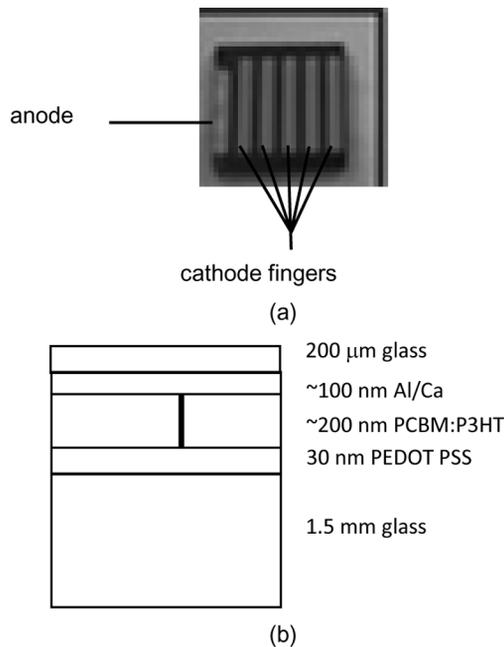
Fig. 2. (a) A picture of one of solar cells ( $1.5 \times 1.5$  cm) studied. (b) A schematic drawing of the cross section below a cathode finger of solar cells studied. The single thick line represents the active region simulated by the modeling.
