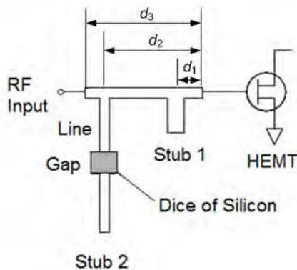
Fig. 3 Schematic of the reconfigurable input matching network
