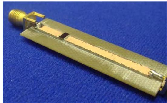
Fig. 1 A Silicon switch in a microstrip transmission line
