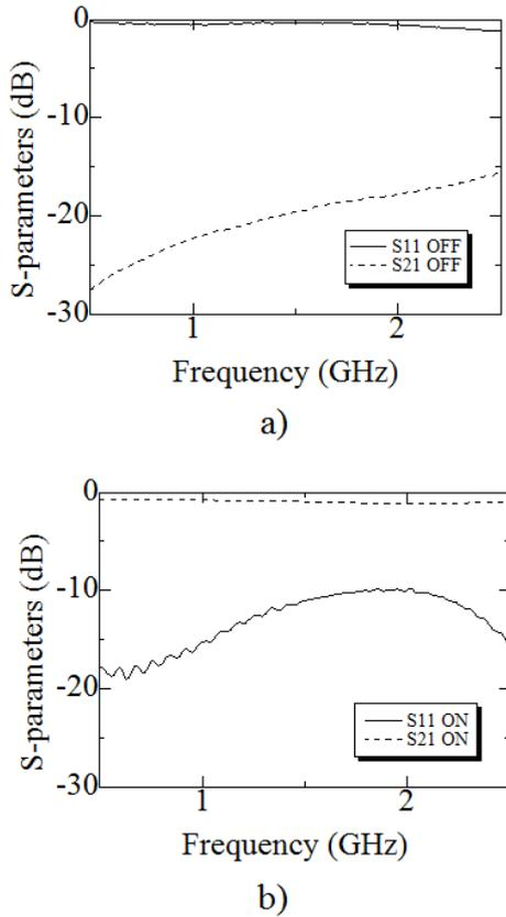
Fig. 2 Measured S-parameters magnitude response for the switch
