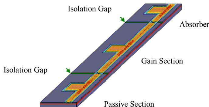
Fig 1, 3-Section Quantum Dot Passively Mode-Locked Laser Device Layout
