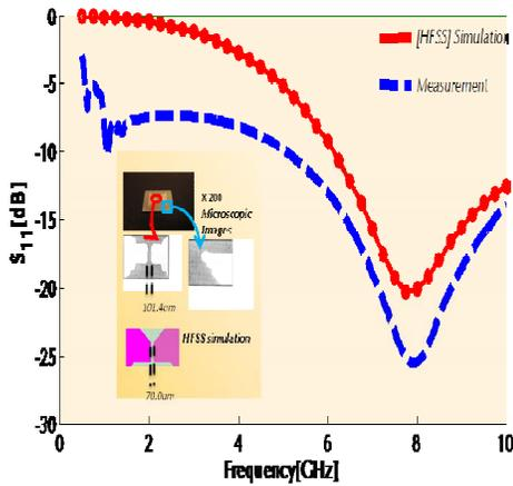
Fig 6, Comparison of simulated and measured  $S_{11}$  with exposure time of 10sec and development time of 30sec.
