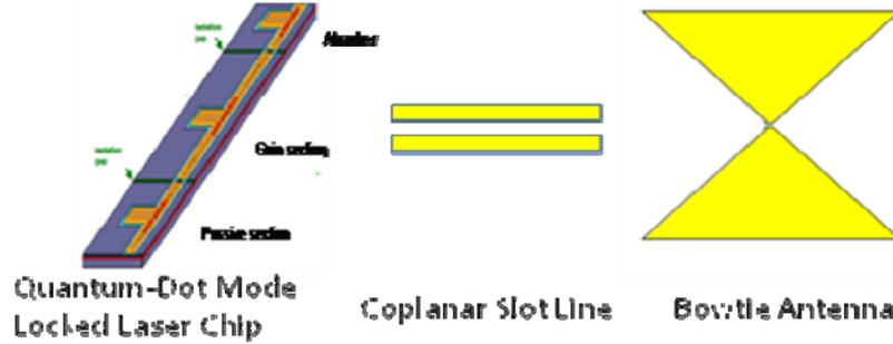
Fig 2, Schematic of the QD-MLL coupled bowtie antenna
