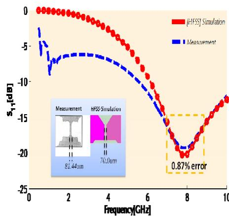
Fig 7, Comparison of simulated and measured  $S_{11}$  for exposure time of 50sec and development time of 35sec.
