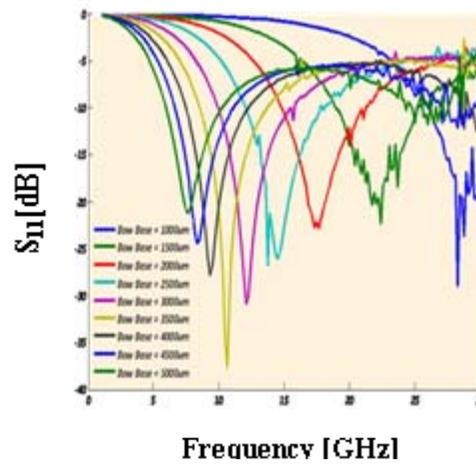
Fig 4,  $S_{11}$  of bowtie antenna as a function of operating frequency for various bow lengths
