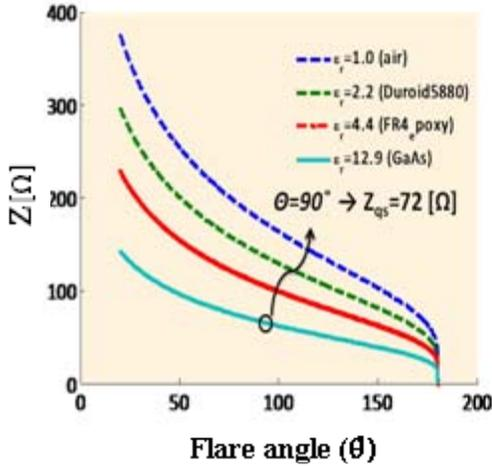
Fig 3,  $Z_{qs}$  as a function of the antenna flare angle for different substrates
