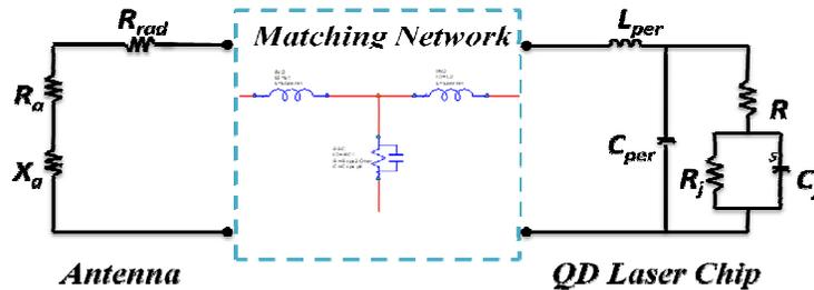
Fig 5, Equivalent circuit model
