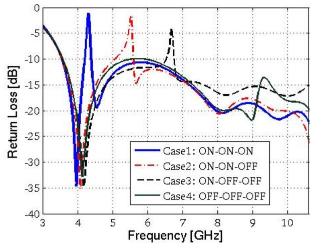
Fig. 4. Simulated return loss of Design A
