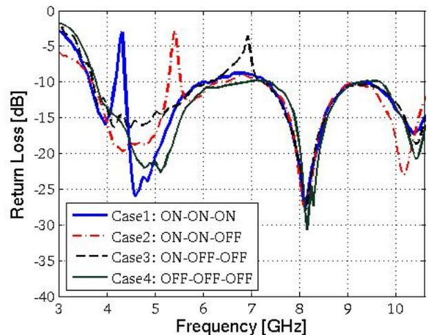
Fig. 5. Measured return loss of Design A
