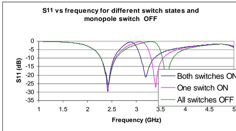
Figure 4.  $S_{11}$  versus frequency when monopole switch OFF for  $L_4=0.5$  mm and  $L=12$  mm
