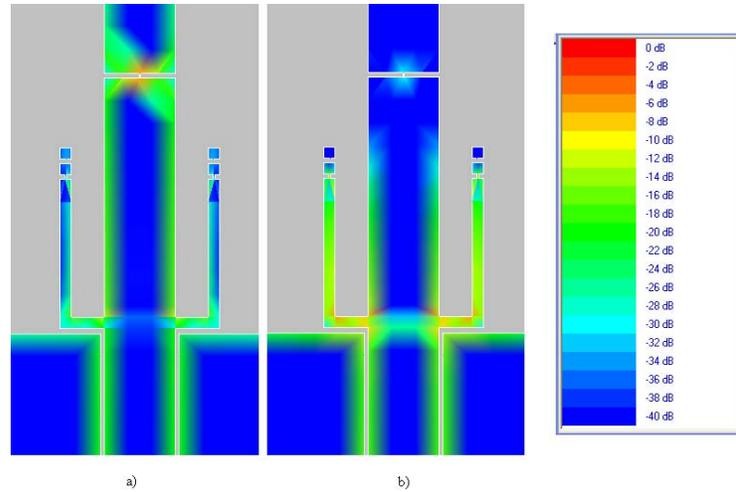
Figure 3. a) Surface currents at  $f_1=1.85$  GHz and b) surface currents at  $f_2=3.4$  GHz for the case of monopole switch ON and only one sleeve switch ON
