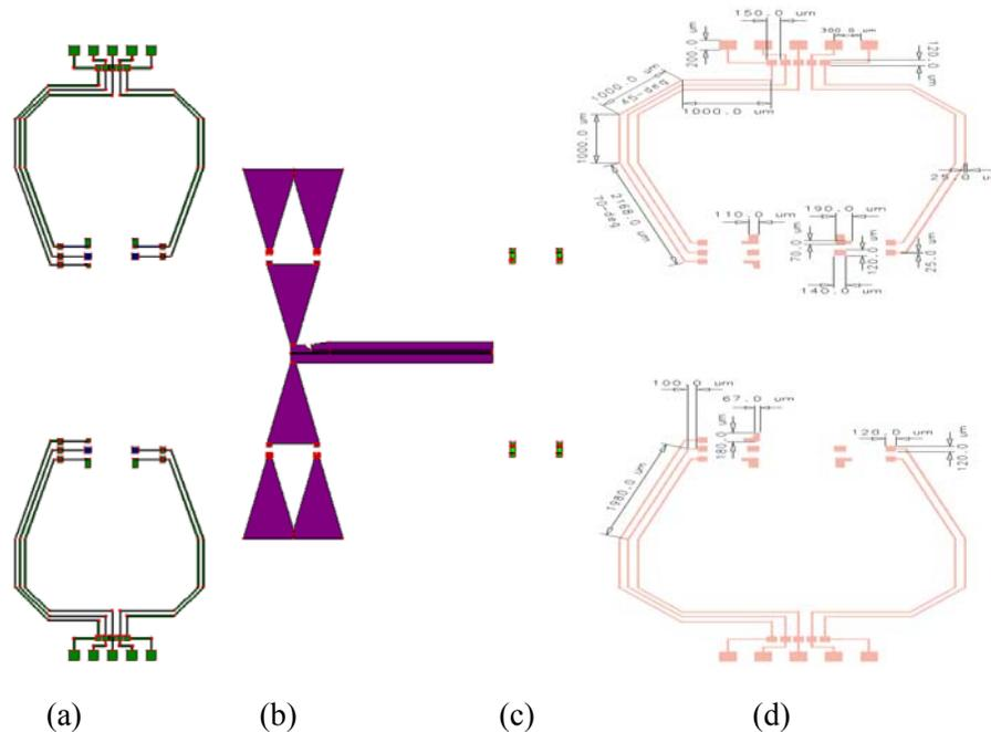
Figure 5. a-c) Different layers of the layout of the antenna. Wire bonding and the small metal connections of the switches to the biasing electrodes are not included. d) Basic dimensions of
