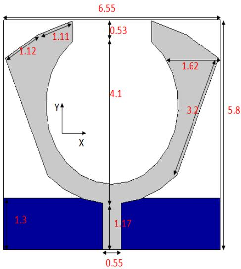
Figure 4 The wideband antenna structure with its dimensions [6]
