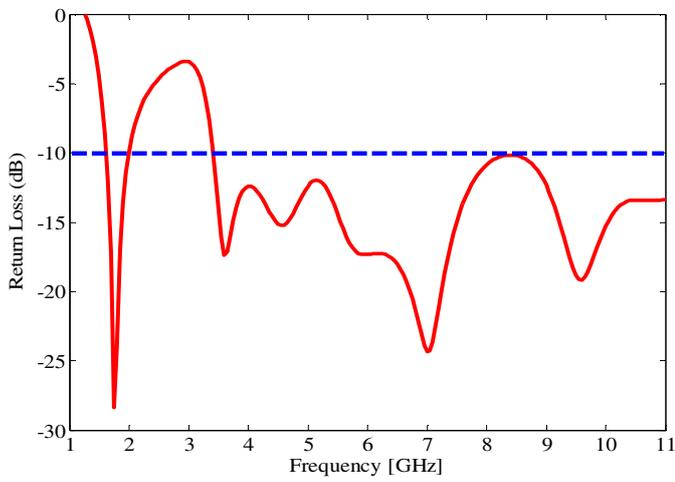
Figure 5 The Wideband Antenna's reflection coefficient
