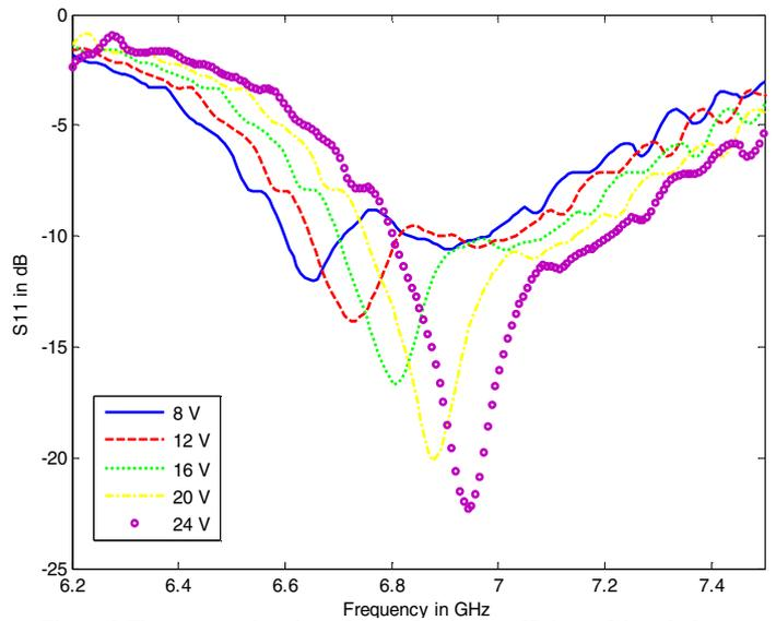
Figure 9 The measured tuning of the reflection coefficient of the whole antenna system showing tunable filtering.
