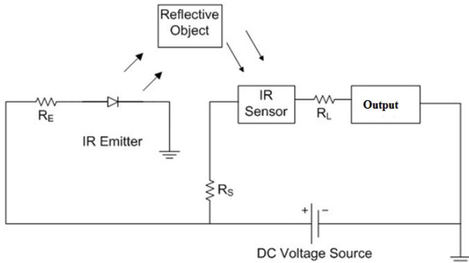
Figure 1 IR circuit Block Diagram
