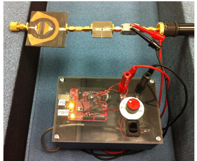
Figure 8 The measurement setup for the whole antenna filter system
