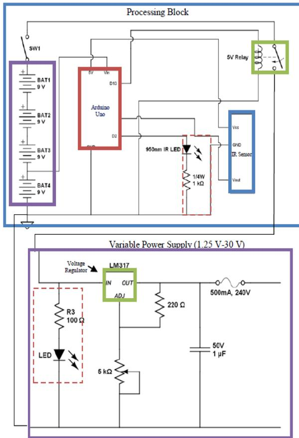
Figure 2 IR Circuit Diagram
