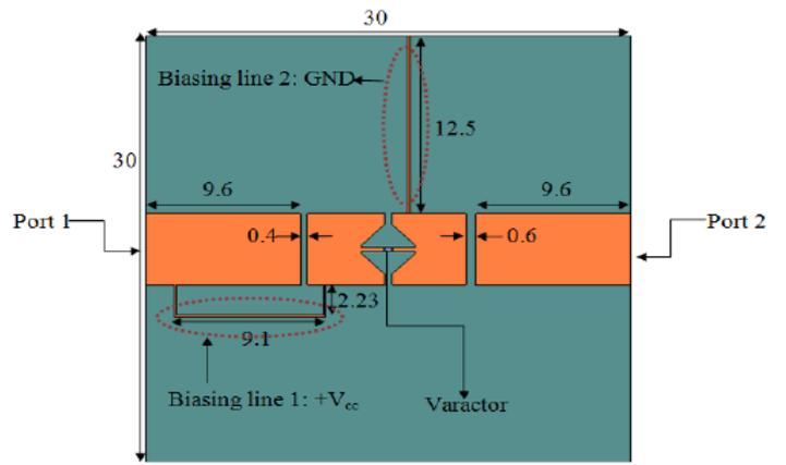
Figure 7 The reconfigurable filter structure [5]
