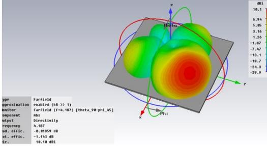
Figure 2. Main beam at  $\theta = 90^\circ$  and  $\phi = 45^\circ$ .
