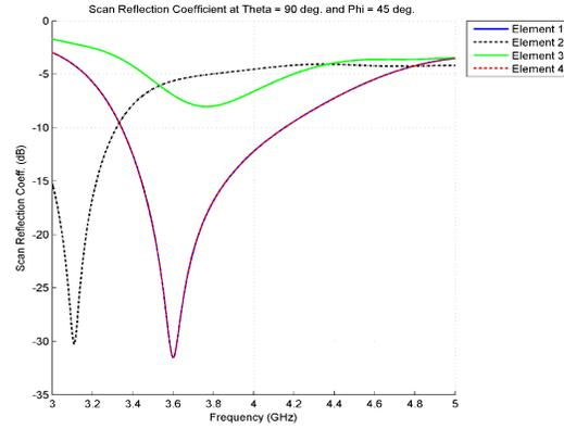
Figure 3. CST MWS Scan Reflection Results
