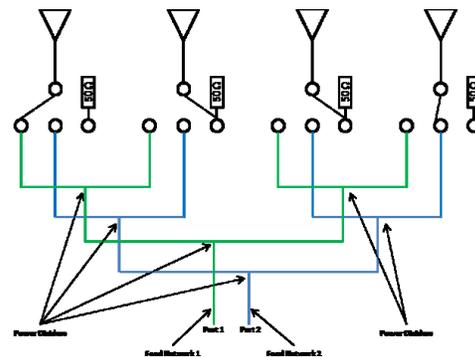
Figure 1. In-Situ mutual coupling measurement system, example configuration.
