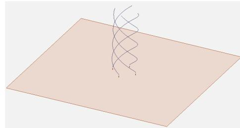
Fig. 1 Quadrifilar Helix Antenna with Ground plane.
