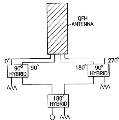
Fig.4 Feeding network of the quadrifilar helix antenna [4]
