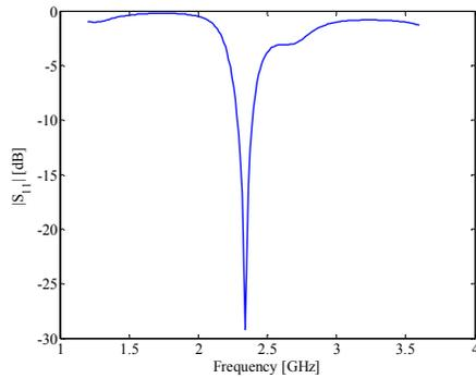
Fig.2 Reflection coefficient showing operation at 2.34 GHz
