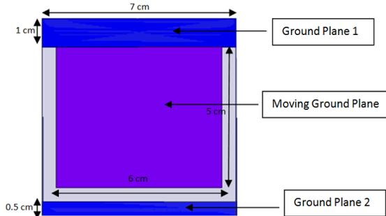
Fig.2 The antenna's bottom layer with the dimensions of the different ground planes.
