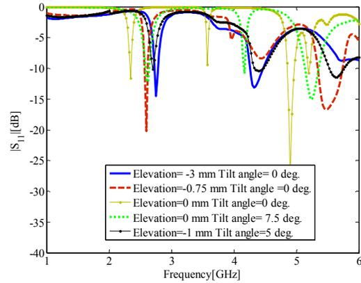
Fig.4 Tuning of Antenna frequency response for various ground position and tilt angles
