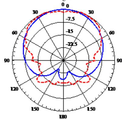
Fig.5 Comparison between measured and simulated radiation pattern in the  $x-z$  plane for  $F=2.4$  GHz, Elevation=0 mm, Tilt angle=0 deg
