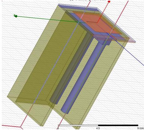
Fig.3 The whole antenna systems with rail and chassis as included in Ansys HFSS simulation
