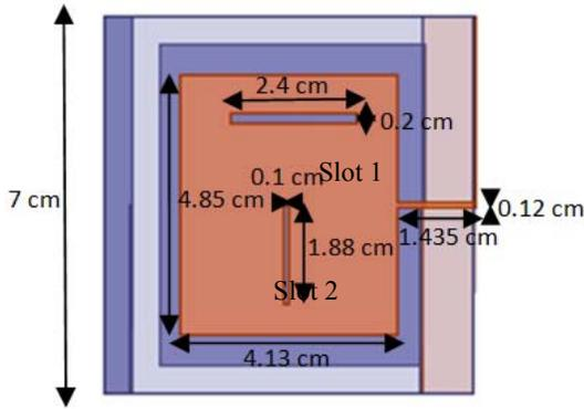
Fig.1 The antenna's top layer with its dimensions
