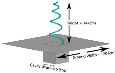
Fig.2 Antenna Deployed with Cavity and dimensions
