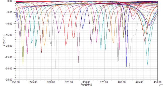
Fig.4 The frequency tuning shown in the antenna's reflection coefficient for various positions
