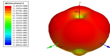
Fig.5 Radiation pattern of the helical antenna throughout its operation
