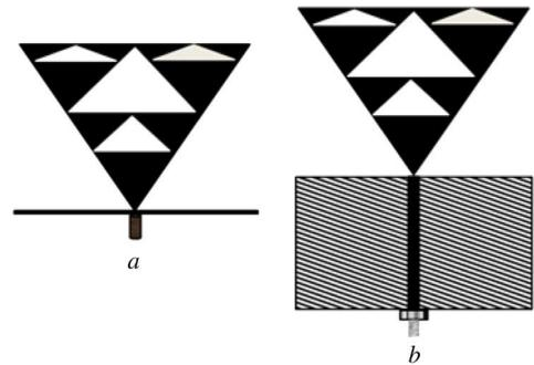
Fig. 1. Feeding to Sierpinski gasket: (a) classical and (b) modified feeds.
