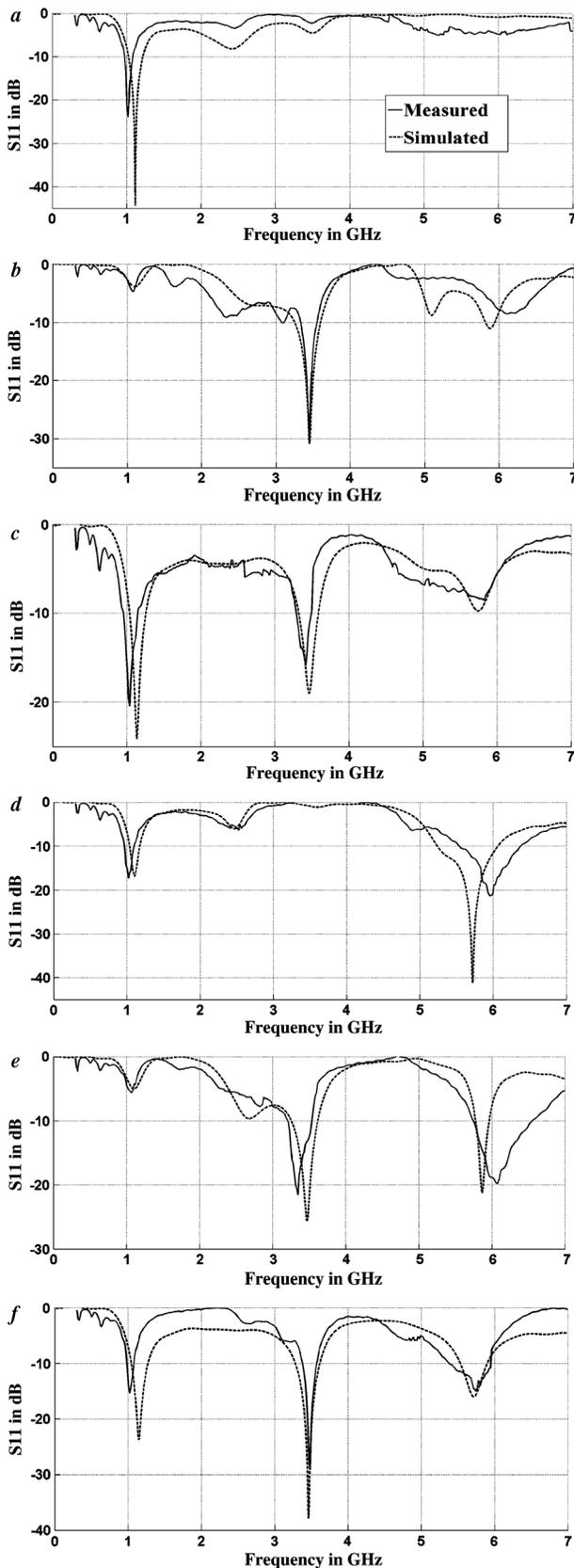
Fig. 4.  $S_{11}$  plots of some typical single- and multiple-resonance behavior of the reconfigurable antenna.
