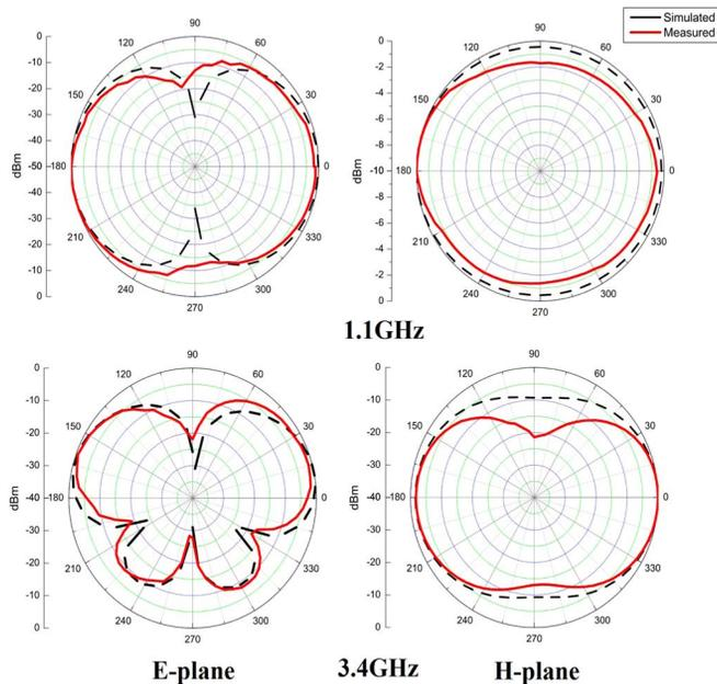
Fig. 6. Radiation patterns at the two working frequencies corresponding to typical case (c).
