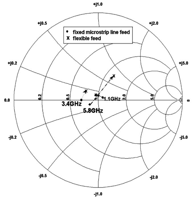
Fig. 5. Smith chart showing shift of the impedances for the three frequencies for a typical case (c) of the flexible feed with respect to the fixed microstrip line feed.
