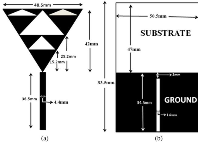
Fig. 2. Design dimensions on the (a) front and (b) back view of the antenna.
