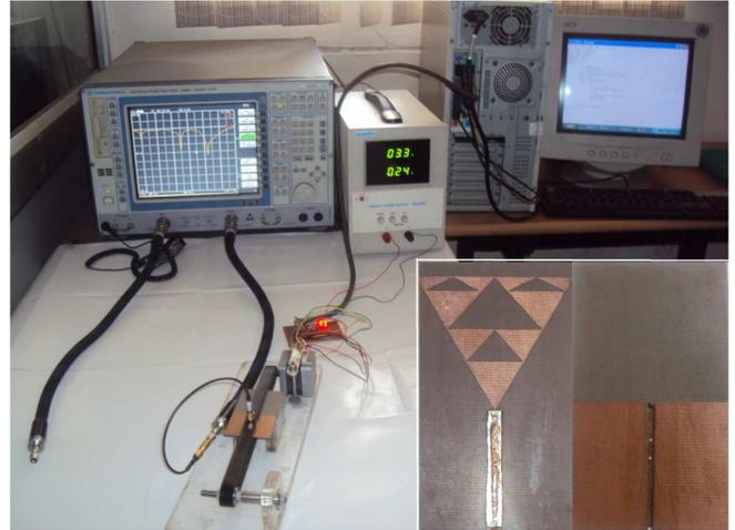
Fig. 3. Photograph of the reconfigurable feeding and measurement setup with the front and back views of the antenna in the inset.
