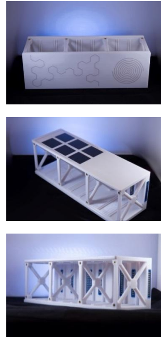
Figure 1. 3D-printed polymer 3U CubeSat.
