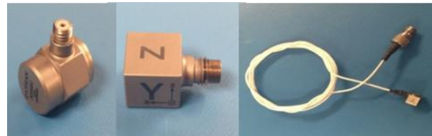
Figure 4. Dytran accelerometers used in the demonstration.
