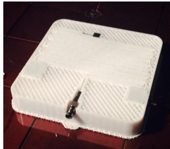
(b) 3D-printed caps installed above larger sensors.
