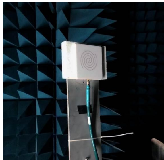
Figure 12. The printed spiral undergoing pattern measurement in the far-field antenna range at NASA Glenn Research Center.
