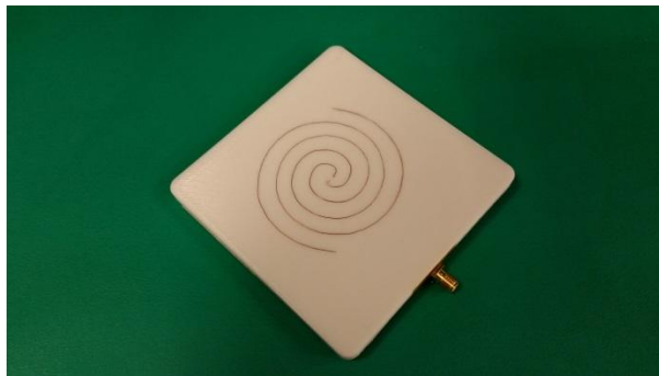
Figure 11. An embedded two-arm Archimedean spiral.
