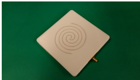
Figure 6. An S-band planar 2-arm Archimedean spiral printed into a 10cm x 10cm polycarbonate plate.
