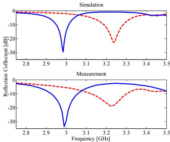
Figure 2. The comparison between the simulated and the measured antenna reflection coefficient when “ $\{S_{1, Left}\}$  OR  $\{S_{2, Left}\}$  are ON (red dotted curve)” and when “ $\{S_{1, Left}, S_{2, Left}\}$  OR  $\{S_{1, Right}, S_{2, Right}\}$  are ON (blue solid curve)”
