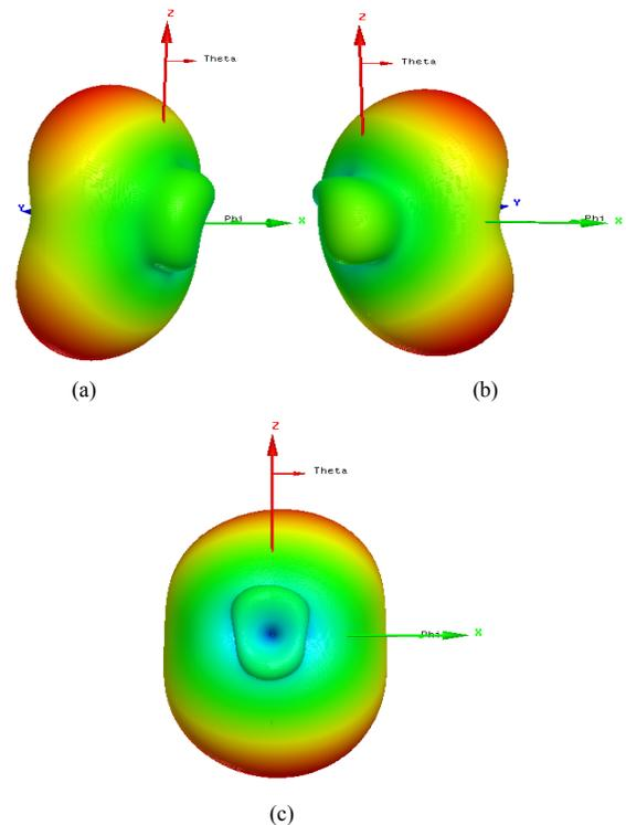
Figure 3. The 3D antenna radiation pattern at  $f=3.25$  GHz when (a)  $S_{1, Left}$  is ON (b)  $S_{1, Right}$  is ON (c) both are ON
