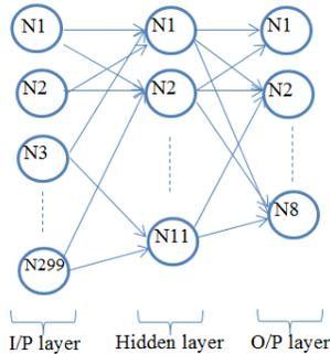
Figure 2. The NN modeling of the frequency reconfigurable antenna array
