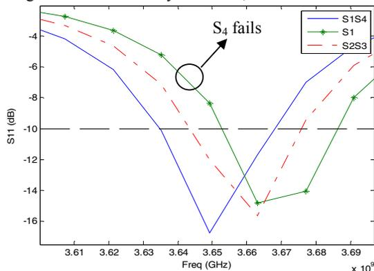
Figure 3. The equivalent configurations for the frequency reconfigurable antenna array at  $f=3.65$
