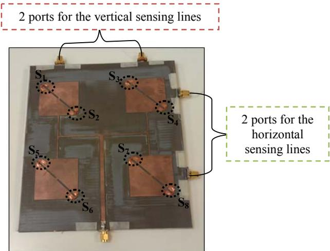
Figure 1. The frequency reconfigurable antenna array
